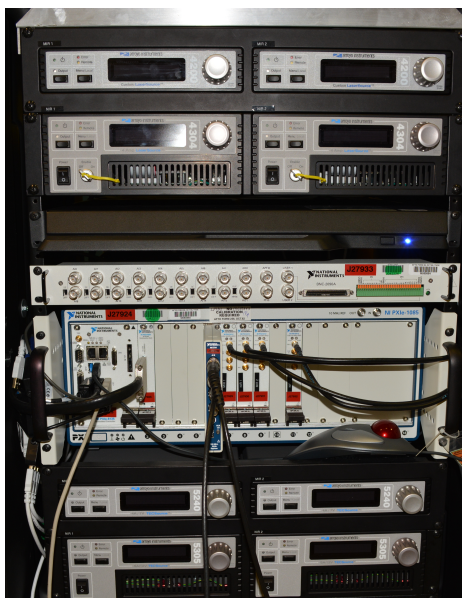
Figure 3.2: The rack mounted laser drivers and Thermo-Electric Coolers (TECs) that control the lasers in the experiment. The experiment was originally planned for four lasers; however, only two lasers were used. The top two laser drivers were the drivers in use, and the bottom two TECs were the TECs in use.
